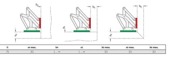
The design variants shown represent standard installation conditions. If the installation position of the hinge is changed or one of the two wall thickness dimensions is lower than s or b, the maximum achievable dimensions change independently of each other. This makes it possible in some cases to work with larger wall thickness dimensions than those specified with the same hinge size. A simple design check via CAD or a test setup is therefore recommended.
